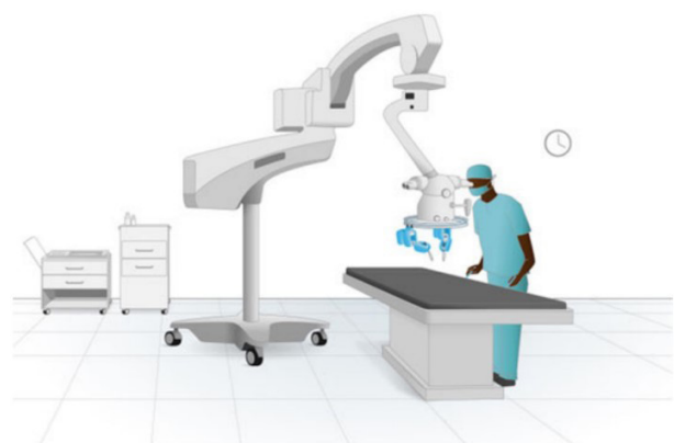
Figure 2. Schematic set up of the Microsure Tobot. The system can be attached to a surgical microscope or the operation table. 32
